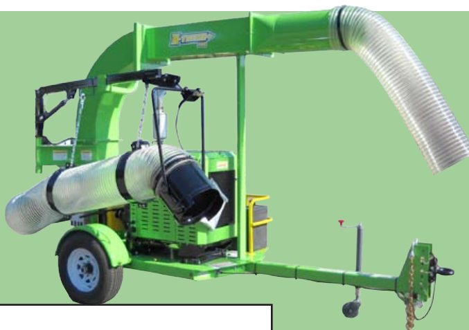
Customized, modular sheet metal with louvers is provided to protect the engine while allowing access to all the critical maintenance areas.
