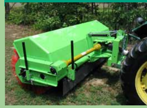
Heavy Duty Hood and Rubber Curtain protects the operator from dust
