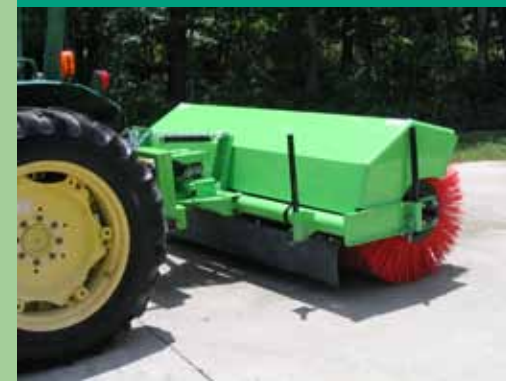
Heavy Duty Hood and Rubber Curtain protects the operator from dust
