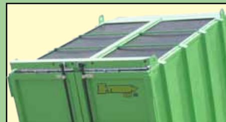
Vented top screens are located on top of the unit for proper air flow. These screens are made of 1/2" expanded steel with mesh screen. They are easily removable and slide in and out on channels.
